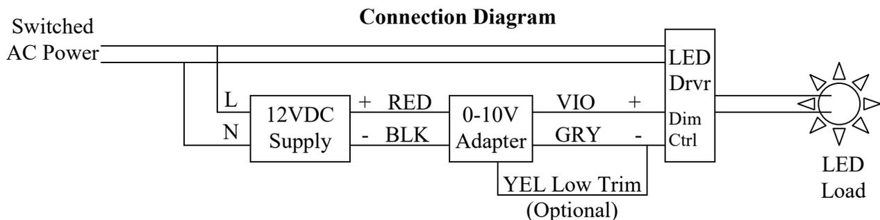
**0-10V Control Signal Out:** Connect the violet(+) and gray(-) wires of your adapter to the respective + and - 0-10V Control terminals of your fixture(s). In most cases the fixture 0-10V Control connections will be wires of like colors. Consult your fixture documentation to be sure.
